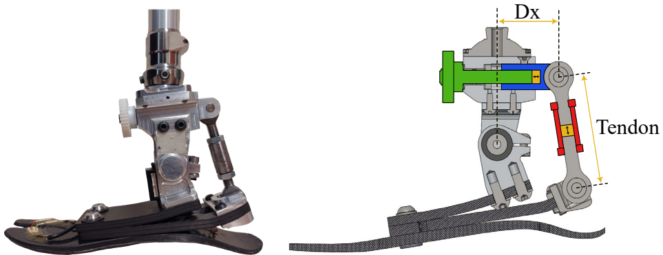
Figure 7.1: Left: The prosthetic foot MyFlex- \eta with tunable stiffness and tunable alignment [10-12]. Right: A schematic representation. The stiffness and alignment of the prosthetic foot depend on the Dx-length and the tendon length. The Dx-length could be changed by manually turning the knob (green), horizontally translating the position of the Dx-slider (blue) (note that a change in Dx-length affects the alignment as well). The orientation of the foot plate relative to the pylon could be changed by turning the threaded tube adaptor (red) of the tendon link that modifies the tendon length.
