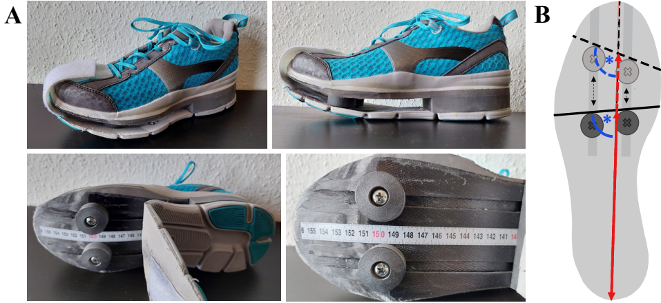
Figure 3.1: A) Experimental shoes with adjustable apex position and apex angle. The position of the cylinders (bottom) could be changed across the rails, by manually screwing the bolts. B) Displayed how changing the cylinders results in a new (dashed) apex position (red) and apex angle (blue asterisk).
